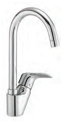
RAK17050-01 Single Lever Sink Mixer DN-15 Swivelling U Spout Ceramic Cartridge: K35 PCA Aerator M 22 x 1 1/2" High Pressure Flexible Hose with PEX Tubes European Standard: EN 817
