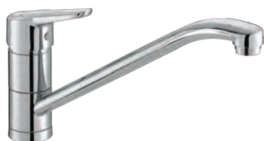
RAK11010-01 Single Lever Sink Mixer DN-15 Ceramic Cartridge: K35 Swivelling: 360°, Spout L-260 mm Aerator: M 24 x 1 1/2" High Pressure Flexible Hose with PEX Tubes European Standard: EN 817
